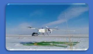
Secure hardware backup Dual redundant airspeed meter/satellite, three redundant heading measurement, four redundant IMUs
